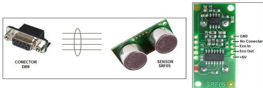
**Figura 0.3 Sensor SRF05 y conector DB9 hembra**
