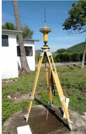
Figura 3.15. Receptor GPS RTK
