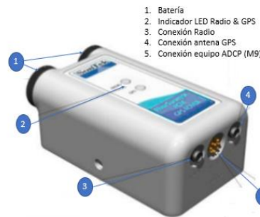
Figura 3-34. Módulo PCM (power & Communication)
