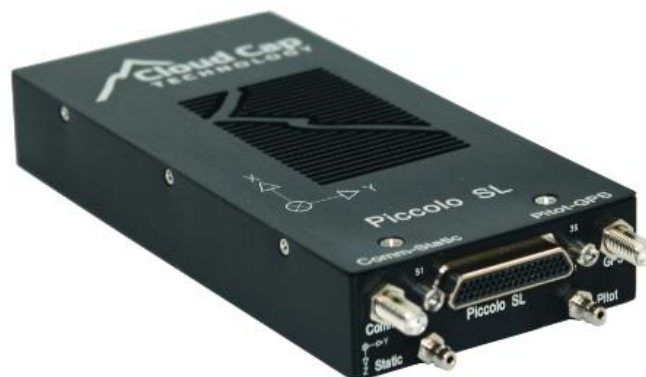
Figura 3.2 Autopiloto de Cloud Cap Technology (Barton, 2012)
