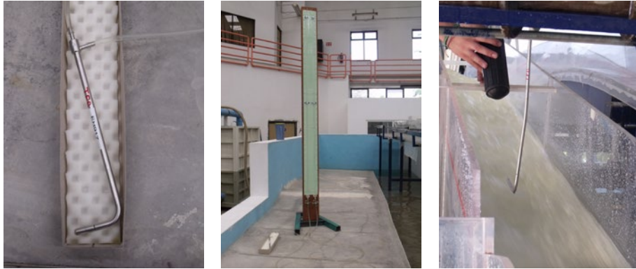
Fig. C.1. Pitot tube: (a) instrument, (b) water manometers and (c) laboratory testing.
